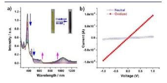
**Figure 8.** (a) UV titration upon adding NOBF<sub>4</sub> solution to a solution of  $HTC_{Gemini}$  in  $CH_2Cl_2$  (1 mM); (b) *I*–*V* curve of a device fabricated from the nanofibers of  $HTC_{Gemini}$  before and after oxidation with NOBF<sub>4</sub> at 25 °C.
